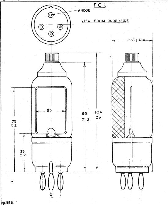
I. THE PORTION OF THE GLASS WALL OPPOSITE THE ANODE WHICH IS COVERED BY THE PHOTOELECTRIC LAYER SHOULD COMPRISE AT LEAST THE AREA BOUNDED BY THE PROJECTION OF THE ANODE LOOP ON THE GLASS WALL OF THE CELL IN THE DIRECTION PERPENDICULAR TO THE PLANE OF THE ANODE LOOP.
