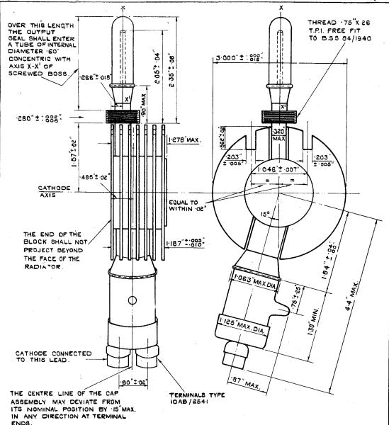
NOTE: TO ENSURE INTERCHANGEABILITY OF SINGLE AND DOUBLE FILAMENT STEM VERSIONS OF CV 208, THE APERTURE IN THE HOUSING, FOR THE FILAMENT SEAL SHOULD CLEAR AN ELIPTICAL CYLINDER CONCENTRIC WITH AXIS OF FILAMENT STEM ASSEMBLY, HAVING MAJOR AXIS OF 1:25" PARALLEL TO AXIS OF CATHODE AND MINOR AXIS OF 1:063" IN A PLANE PARALLEL TO THE RADIATOR FINS. IF THE HOUSING DOES NOT SPLIT, THE DESIGNER SHOULD EXAMINE BOTH CV 208 DRAWINGS AND THE DRAWING IN SPECIFICATION CV 209
