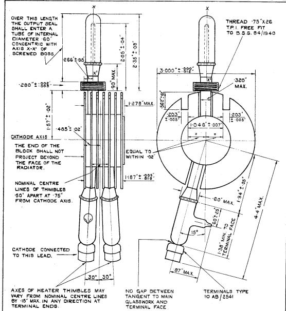
NOTE - TO ENSURE INTERCHANGEABILITY OF SINGLE AND DOUBLE FILAMENT STEM VERSIONS OF CV208, THE APERTURE IN THE HOUSING, FOR THE FILAMENT SEALS SHOULD CLEAR AN ELIPTICAL CYLINDER CONCENTRIC WITH AXIS OF FILAMENT STEM ASSEMBLY, HAVING MAJOR AXIS OF 1:25" PARALLEL TO AXIS OF CATHODE AND MINOR AXIS OF 1:063" IN A PLANE PARALLEL TO THE RADIATOR FINS IF THE HOUSING DOES NOT SPLIT THE DESIGNER SHOULD EXAMINE BOTH CV208 DRAWINGS AND THE DRAWING IN SPECIFICATION CV 209.
