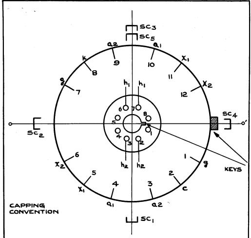
WHEN VIEWING THE TUBE FACE WITH KEYS OF THE TUBE AT 9.0'CLOCK THEN A POSITIVE VOLTAGE APPLIED TO SC3 SHALL DEFLECT THE BEAM OF GUN I UPWARDS.
