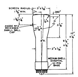
C OF BULB WILL NOT DEVIATE MORE THAN 20 IN ANY DIRECTION FROM PERPENDICULAR ERECTED AT THE CENTER OF BOTTOM OF BASE.
