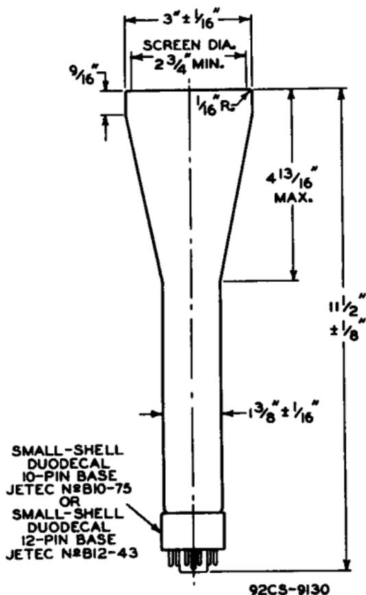
CL OF BULB WILL NOT DEVIATE MORE THAN  $2^\circ$  IN ANY DIRECTION FROM PERPENDICULAR ERECTED AT CENTER OF BOTTOM OF BASE.
