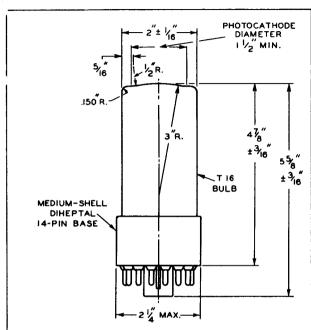
$\ensuremath{\mathbb{Q}}$  of bulb will not deviate more than  $2^{\ensuremath{\text{O}}}$  in any direction from the perpendicular erected at the center of bottom of the base.
