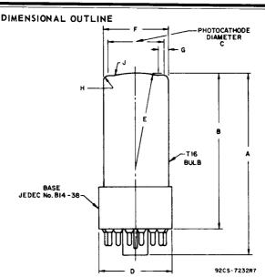
$\[ \[ \varphi \]$  of bulb will not deviate more than  $2^{\[ O \]}$  in any direction from the perpendicular erected at the center of bottom of the base.
