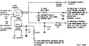
\* The value of this capacitor should be such that its charging time constant is at least five times greater than the firing time of the spark gap..
