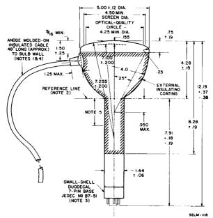
Note 1: The plane through the tube axis and vacant pin position No.3 may vary from the plane through the tube axis and anode-cable connection at bulb wall by angular tolerance (measured about the tube axis) of  $\pm 20^{\circ}$ . Anode-cable connection is on same side as vacant pin position No.3
