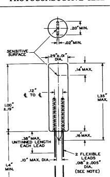
NOTE: THE SPECIFIED LEAD DIAMETER IS MAINTAINED ONLY WITH-IN THE UNTINNED LENGTH.
