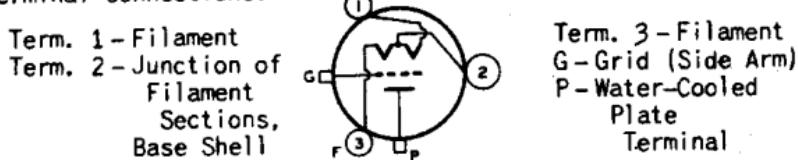
Mounting Position . . . . . Vertical, Filament End Up
