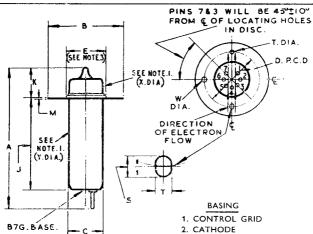
NOTE. 1. THIS PORTION OF BULB WILL NOT FOUL A CYLINDER OF INT. DIA. SPECIFIED WHICH IS CONCENTRIC WITH THE PITCH CIRCLE OF THE LOCATING HOLES IN THE DISC.
