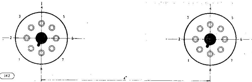
Fig. 2. Correct orientation and spacing of the valve sockets when the valves are mounted horizontally.
