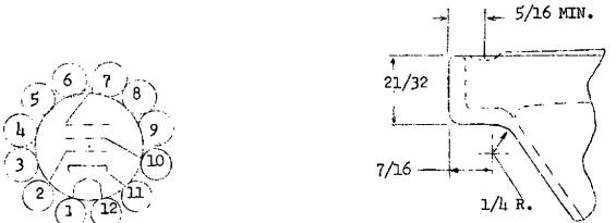
NOTE 1 - REFERENCE LINE DETERMINED BY POSITION WHERE REFERENCE LINE GAUGE #110 WILL REST ON GLASS FUNNEL.
