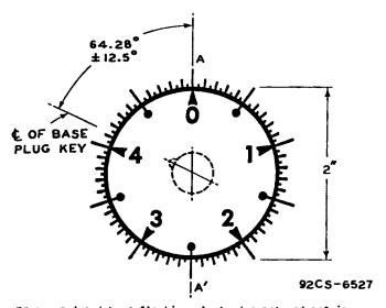
Trace produced by deflecting electrodes DJ1 and DJ2 is along line  $\mathbf{A}\text{-}\mathbf{A}^{*}$  .
