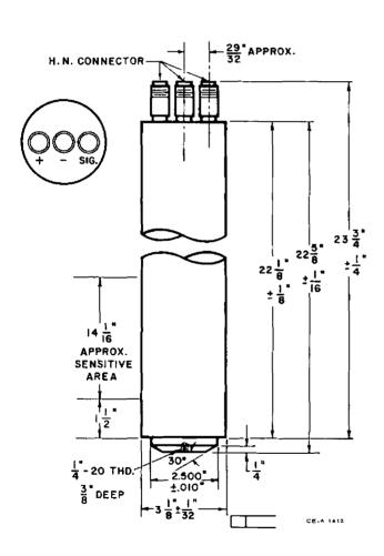
The WL-7353 is electrically similar to the WL-6377. The significant mechanical difference is that the WL-7353 has an extended portion with a tapped hole to facilitate mounting.
