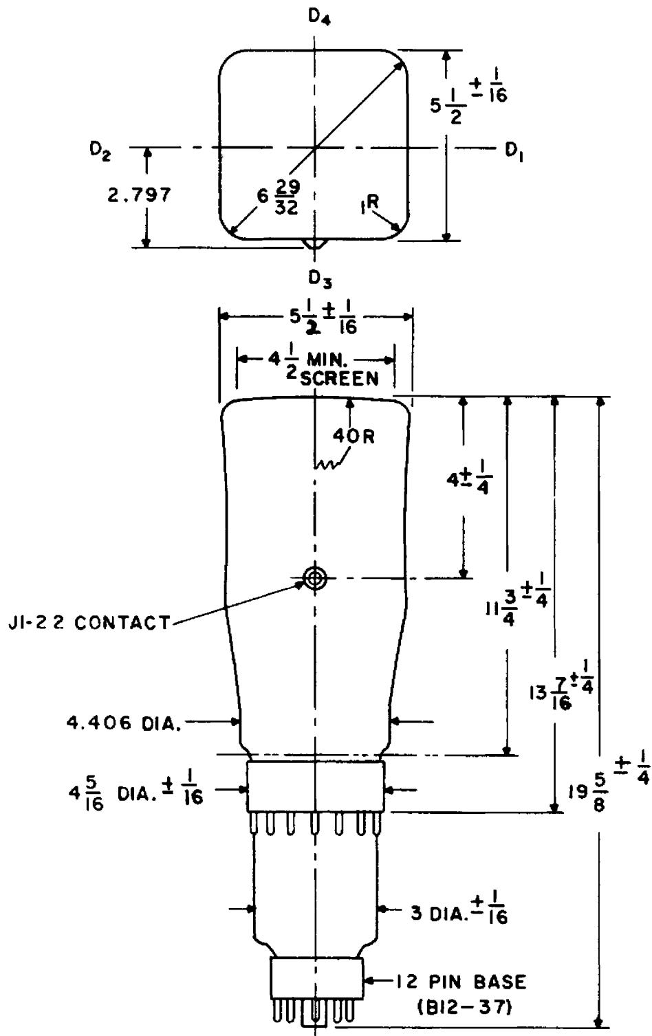
1. COLLAR PINS 4&11 (SHIELD) ARE COMMON TO BOTH BEAMS.
